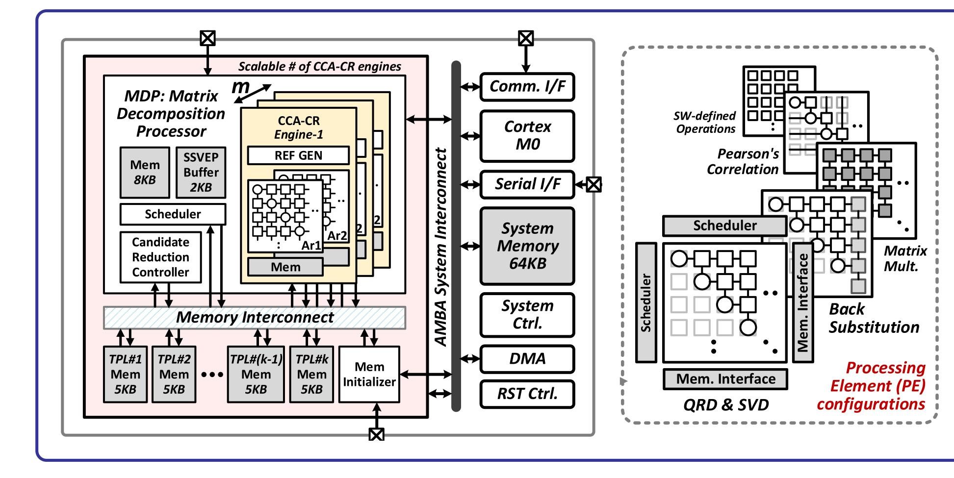
Implementation of proposed CCA-**CR acceleration architecture:** candidate reduction (CR) based optimized CCA-Comb algorithm was proposed and implemented through suitable microarchitecture with 3 **CCA-CR engines (each has 2 arrays)**
